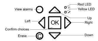
There are seven buttons: 4 arrow buttons which will be called UP, DOWN, RIGHT and LEFT. The menus in the Corrigo E are organized in a horizontal tree structure. The UP / DOWN-buttons are used to move between menus at the present menu level. The RIGHT / LEFT buttons are used to move between menu levels. When changing parameters the UP / DOWN buttons are used to increase / decrease the value of the parameter and the RIGHT / LEFT buttons to move between digits within the parameter.
